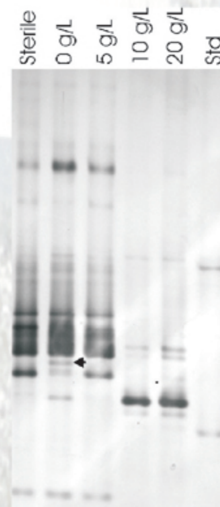
Figure 7. DGGE separation of PCR fragments produced with fungal specific ITS1F and ITS2 primers on DNA extracted from sterilized, non-treated and M. albus treated apple replant soils. DNA bands appearing in the non-treated soil but not in other soils are potential causal agents of apple replant (arrow).
