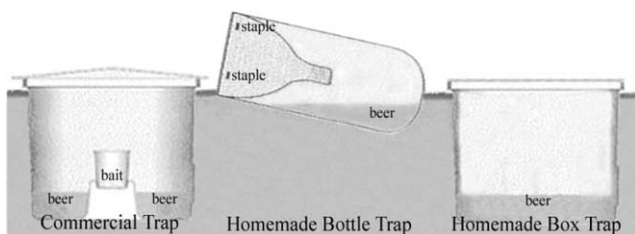
Fig. 1. Construction of the commercial trap, the homemade trap out of a 1.5l PET bottle and the new invented homemade box trap. (Altered from original http://www.odla.nu/artiklar/slugtrap.shtml ; 04-10-08, www.ourgardenpests.com/Traps ; 04-10-08.)
